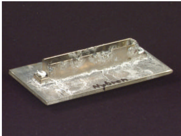
Figure 10 Nybron-plated assembly after salt fog exposure
