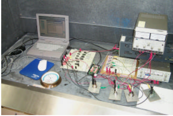
Figure 13 Data acquisition and control interface
